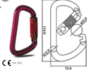
CE EN 362 LX08 Carabiner / Triple Lock Aluminium Alloy MBL: 25kn
